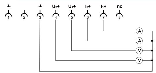
Connection 5: output voltage + strain gauge 1 (0...10 VDC)
