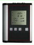
Input: 2 strain gauge full bridges (350 ohms) / Input sensitivity: 0,1...5 mV/V
